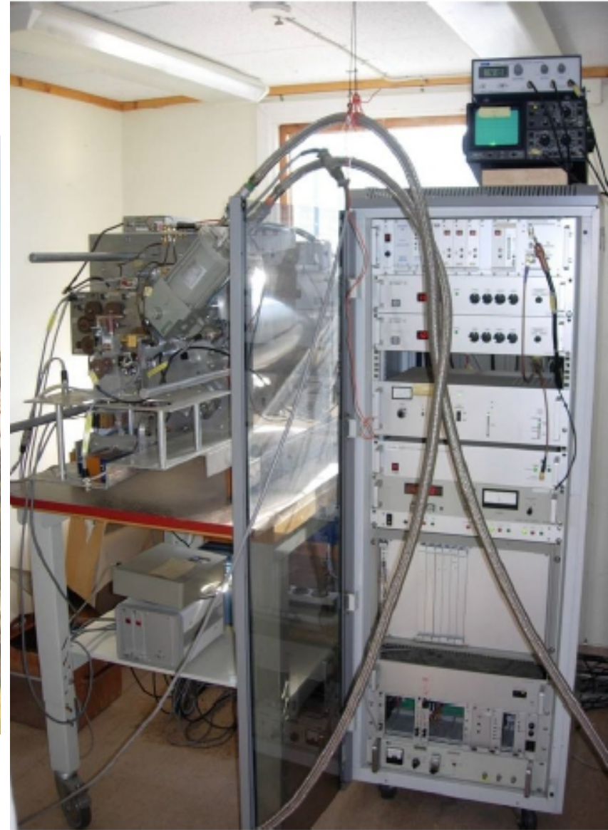
90-120 GHz cooled Shottky SSB mixer
